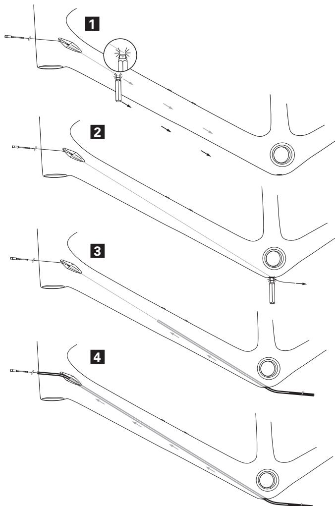
**Method D:** Installing new housing with existing housing.
